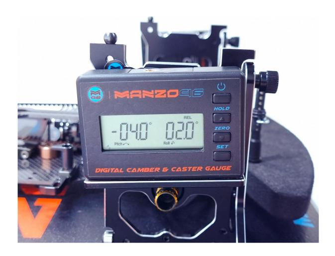
Important to know is when you measure simultaneously on both sides, you have one side of the pitch (caster)in **positive** values and the opposite side on **negative** values. (see in the pictures)
