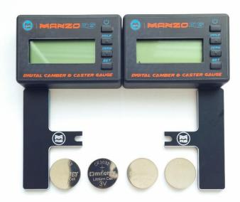
Use a thin double-sided tape (not included) to assemble them with the aluminum parts. Make sure there are no air bubbles under the tape to avoid wrong measurements.
