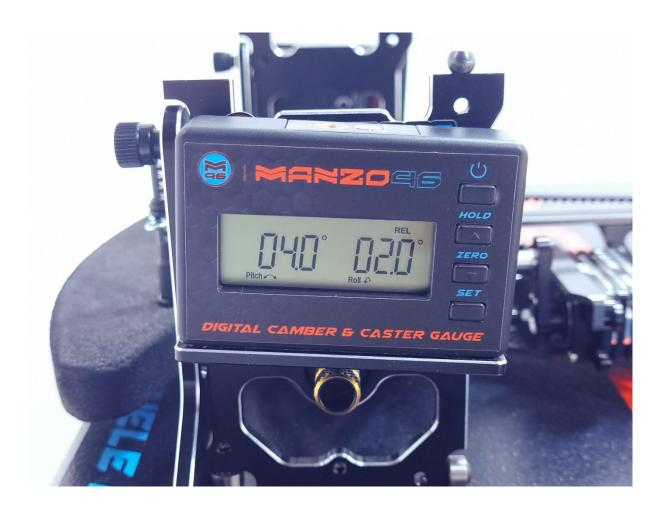
Once the gauges are set on zero you can mount them on your car. The gauge will show you two measurements one is **pitch** (caster) and the other is **roll** (camber).
